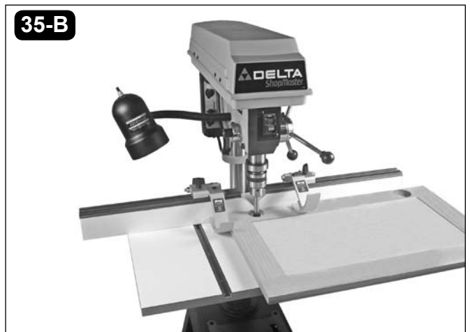
Drilling 35mm holes in door stile for hinge cups.
